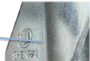
Reinforced wheel ribs, high strength. Bearing cover is nice looking and tight clearance.
